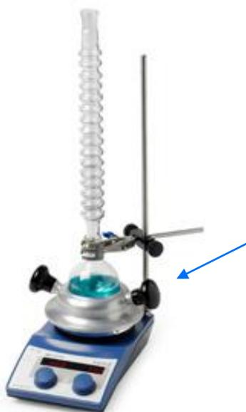
**Figure 9: Image showing a DrySyn heat block in use along with a condensyn air condenser.** DrySyn blocks fit various sizes of round bottom flasks. They eliminate the need of oil and silicon buy in as well as their waste. Furthermore, it takes less energy to heat up a DrySyn block compared to an oil bath to the same temperature. For more info check out our guidelines and benefits booklet.
