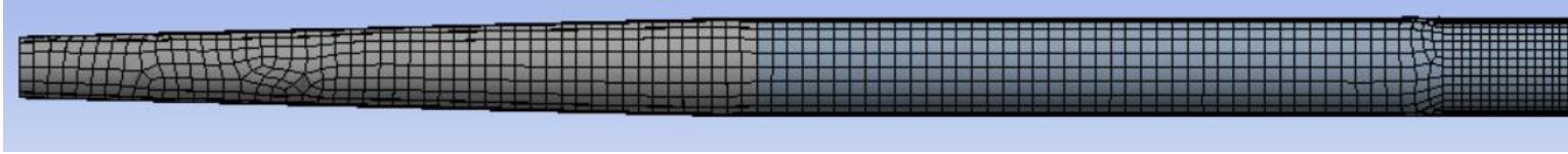
Figure 9 – Example finite element model of wind turbine tower used for finite element analysis [Amiri]
